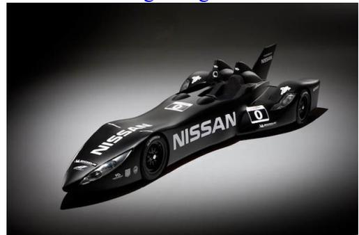
Nissan is supplying the engine for this radical racing car concept which will be unofficially competing in the 24 hours of LeMans endurance race June 16<sup>th</sup>. The engine is derived from the 1.6 liter turbocharged plant found in the Juke. Massaged to 300 bhp, it's significantly less than the 500+ bhp typically found in LeMans race cars, which it makes up for with a body design that is much lighter (1,300 lbs vs !) and has a drag
